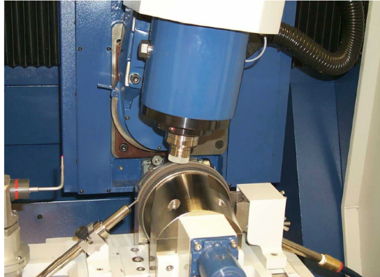
Figure 1.14: Manufacturing of an aspherical lens using a MR process
